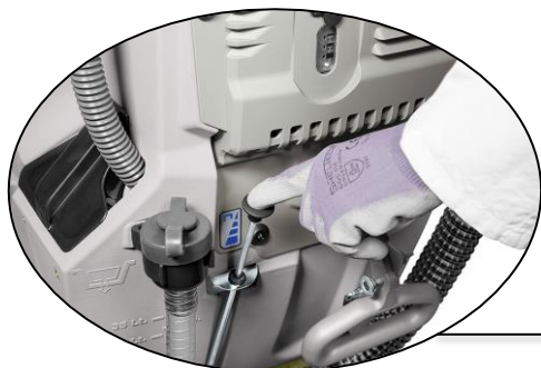
Detergent solution flow adjustment
