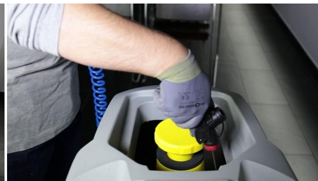
Clean of the recovery tank with a special gun
