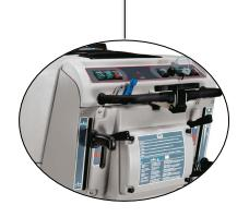
On the machine rear are the controls for lifting and adjusting the scrubbing head as well as the levers for service and parking brakes. There are also two drain plugs on the recovery tank, one being larger for easier internal cleaning.
