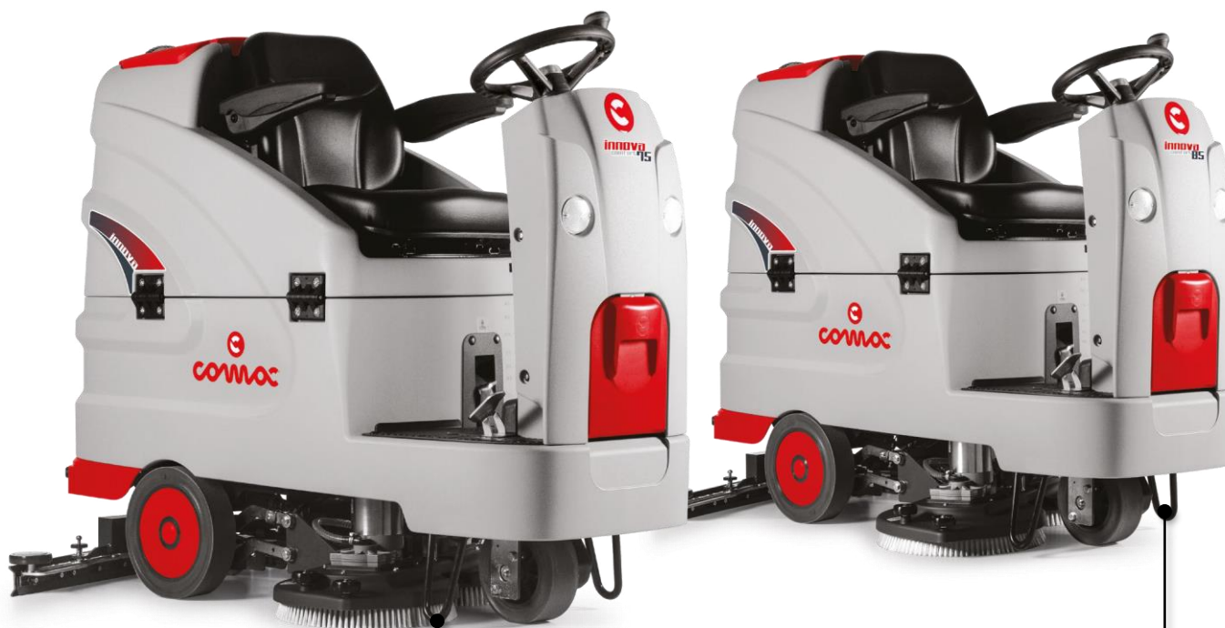
Innova Comfort 75 B Scrubbing version with dual disc brush Working width: 750 mm
